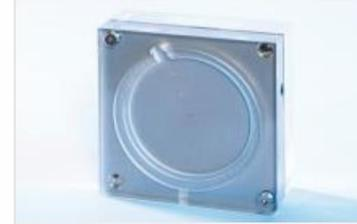
Enhanced Digital Dental QA Test Phantom
