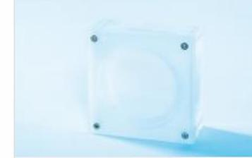
Dental Film-Screen QA Test Phantom
